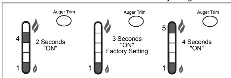
Figure 3: Auger trim and heat level indicator.
